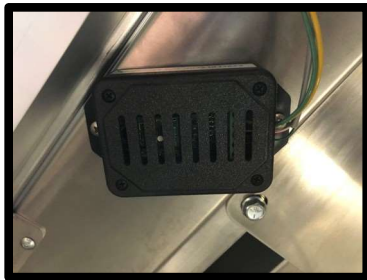
Interior ozone sensor
